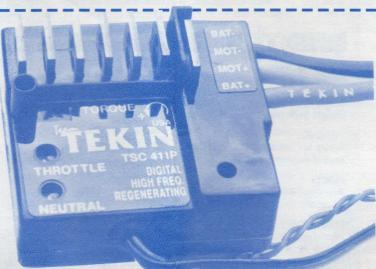
(-) side of the motor. This leaves the positive (+) side of the motor without a connection. Use a separate piece of monster wire (supplied with the TSC 411P) to connect the positive (+) side of the motor to the positive (+) side of the battery.
